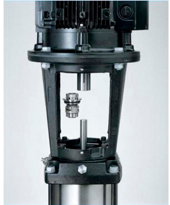
Figure 2: An easily accessible cartridge simplifies mechanical seal replacement for this vertical multistage centrifugal pump in minutes, without having to remove the motor. This avoids the time and effort typically associated with realigning motors and shafts after seal replacement on long-coupled end-suction pumps and split-case pumps.
