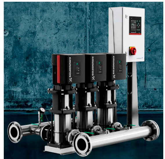
Figure 3: Packaged multipump systems that integrate speed control to ramp throughput up or down quickly can satisfy a broader range of demand with greater energy efficiency than that typically offered by end-suction or split-case pumps.
