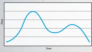
\*Typically, the maximum designed flow is only required for a small percentage of time. High efficiency in part-load conditions is key to saving energy cost.
