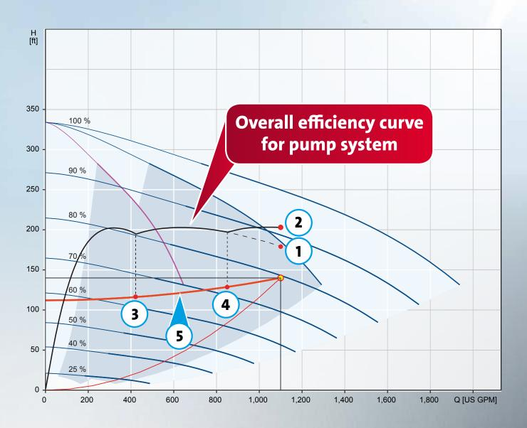
Systems today often use on/off pump solutions based on capacity and do not consider operating efficiency. Operating costs can be optimized by running the most efficient combination of pumps. The figure above, shows how three pumps in operation can reduce the energy at a particular operating point by 12% over two pumps in operation even when two pumps could meet the requirement based on capacity alone.
