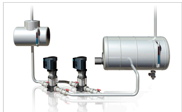
A steam supply with speed-controlled pumps and direct level control in the boiler reduces the number of system components required.
